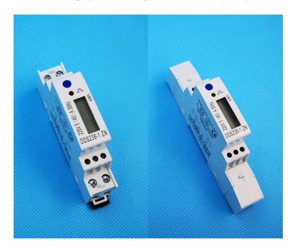
The meter is designed to measure single phase two wire AC active energy like residential, utility and industrial application. It has remote read communication port RS485. It is a long life meter with the advantage of high stability, high over load capability, low power loss and small volume .
