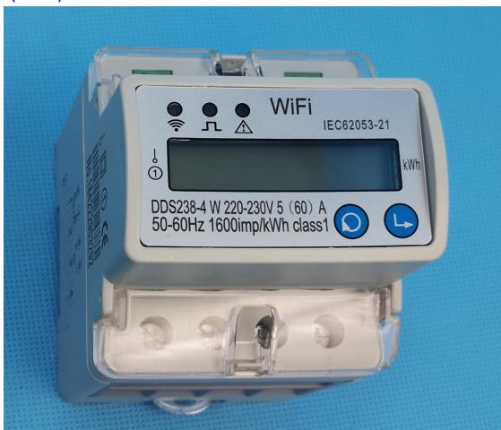
The meter is designed to measure single phase two wire AC active energy variable parameter like residential, utility and industrial application. It has remote read communication port RS485 and WIFI. It is a long life meter with the advantage of high stability, high over load capability, low power loss and small volume.
