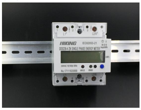
The meter is designed to measure single phase two wire AC active energy with time of use(TOU) function(the power flow of sharp time, peak time, flat time and off-peak time) and variable parameter, it can use for residential, utility and industrial application. It has remote read communication port RS485. It is a long life meter with the advantage of high stability, high over load capability, low power loss and small volume.
