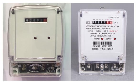
The meter is designed to measure single phase two wire AC active energy. It adopt LSI and SMT technology, the key component are long life international brand product. All of its functions comply with the relative technical requirement for class 1 single phase watt hour meter in IEC62053-21. It is a long life meter with the advantage of high stability, high over load capability, low power loss and compact size.
