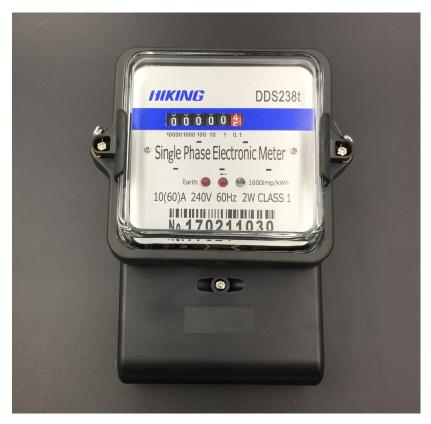
The meter is designed to measure single phase two wire AC active energy. It adopt LSI and SMT technology, the key component are long life international brand product. All of its functions comply with the relative technical requirement for class 1 single phase watt hour meter in IEC62053-21. It is a long life meter with the advantage of high stability, high over load capability, low power loss and anti-tamper function.
