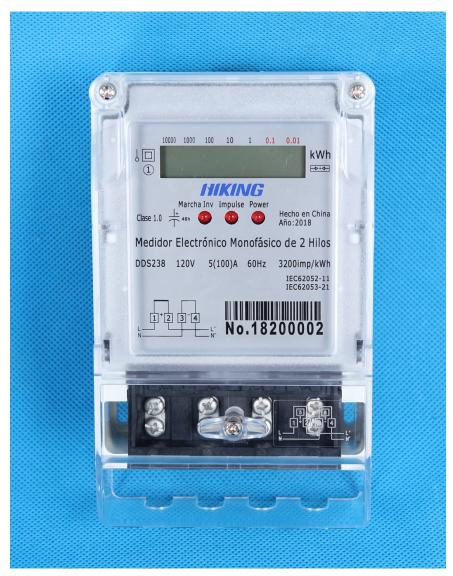
The meter is designed to measure single phase two wire AC active energy for solar system. It adopt LSI and SMT technology, the key component are long life international brand product. All of its functions comply with the relative technical requirement for class 1 single phase watt hour meter in IEC62053-21. It is a long life meter with the advantage of high stability, high over load capability, low power loss and compact size.
