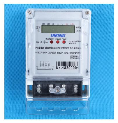
The meter is designed to measure single phase three wire AC active energy in north and south America market. It adopt LSI and SMT technology, the key component are long life international brand product. All of its functions comply with the relative technical requirement for class 1 single phase watt hour meter in IEC62053-21. It is a long life meter with the advantage of high stability, high over load capability, low power loss and compact size.
