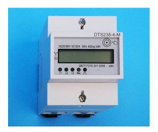
The meter is used in three phase four wire /three phase three wire /two phase three wire power grid. The meter is designed to measure AC active energy. All of its functions comply with the relative technical requirement for class 1 three phase watt hour meter in IEC62053-21. It is a long life meter with the advantage of high stability, high over load capability, low power loss and small volume.
