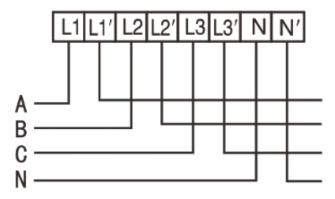
(2) three phase four wire through current transformer connection
