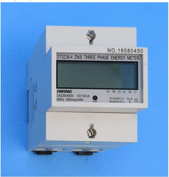
The meter is used in three phase four wire power grid. The meter is designed to measure AC active energy and variable parameter. All of its functions comply with the relative technical requirement for class 1 three phase watt hour meter in IEC61036 and its data communication rules obey the requirement of DL/T645 or MODBUS-RTU. It is a long life meter with the advantage of high stability, high over load capability, low power loss and small volume.
