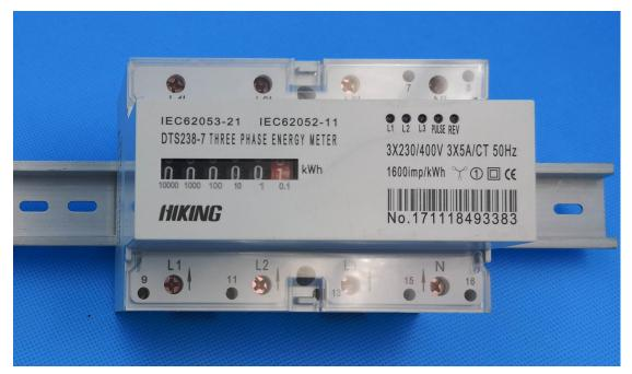
The meter is used in three phase four wire/three phase three wire /two phase three wire power grid. The meter is designed to measure AC active energy. All of its functions comply with the relative technical requirement for class 1 three phase watt hour meter in IEC62053-21. It is a long life meter with the advantage of high stability, high over load capability, low power loss and small volume.
