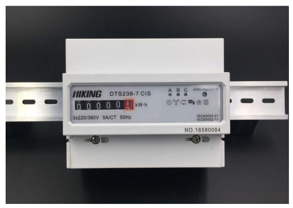
The meter is used in three phase four wire/three phase three wire/two phase three wire power grid. The meter is designed to measure AC active energy. All of its functions comply with the relative technical requirement for class 1 three phase watt hour meter in IEC62053-21. It is a long life meter with the advantage of high stability, high over load capability, low power loss and small volume.
