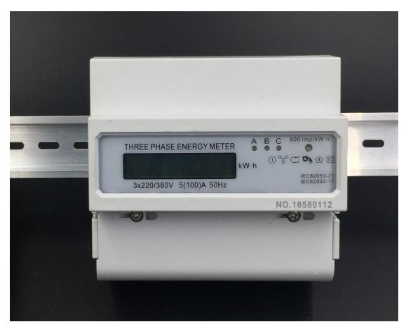
The meter is used in three phase four wire/three phase three wire/two phase three wire power grid. The meter is designed to measure AC active energy. All of its functions comply with the relative technical requirement for class 1 three phase watt hour meter in IEC62053-21. It is a long life meter with the advantage of high stability, high over load capability, low power loss and small volume.
